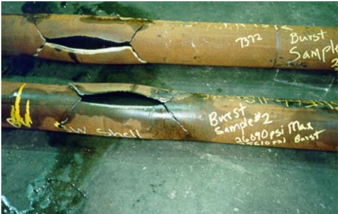
Figure A-2—Brittle Burst Sample
