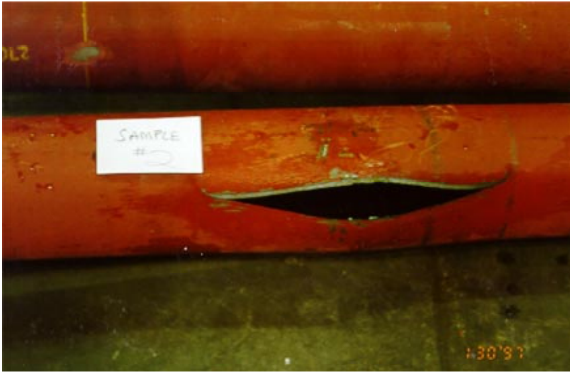
Figure A-1—Ductile Burst Sample
